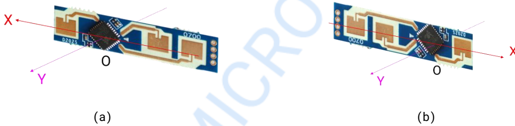
Figure 5-3 Illustration of the coordination system of XenP202TS in recommended poses
